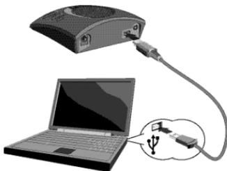
Figure 1. Connecting to a PC
